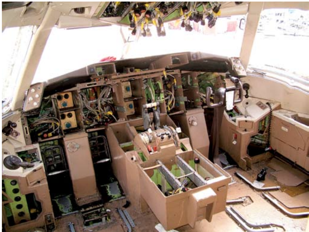
The cockpit was stripped of avionics and parts by ARC and most of the items will find their way into the American fleet.
